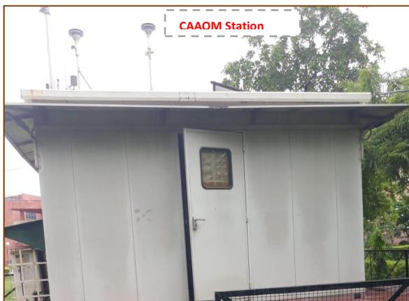
A Continuous Ambient Air Quality Monitoring System is a specialised system equipped for monitoring of ambient air pollutants and transmit the real time data to the Central Server. This data is used for computation of daily National Air Quality Index of the cities.
