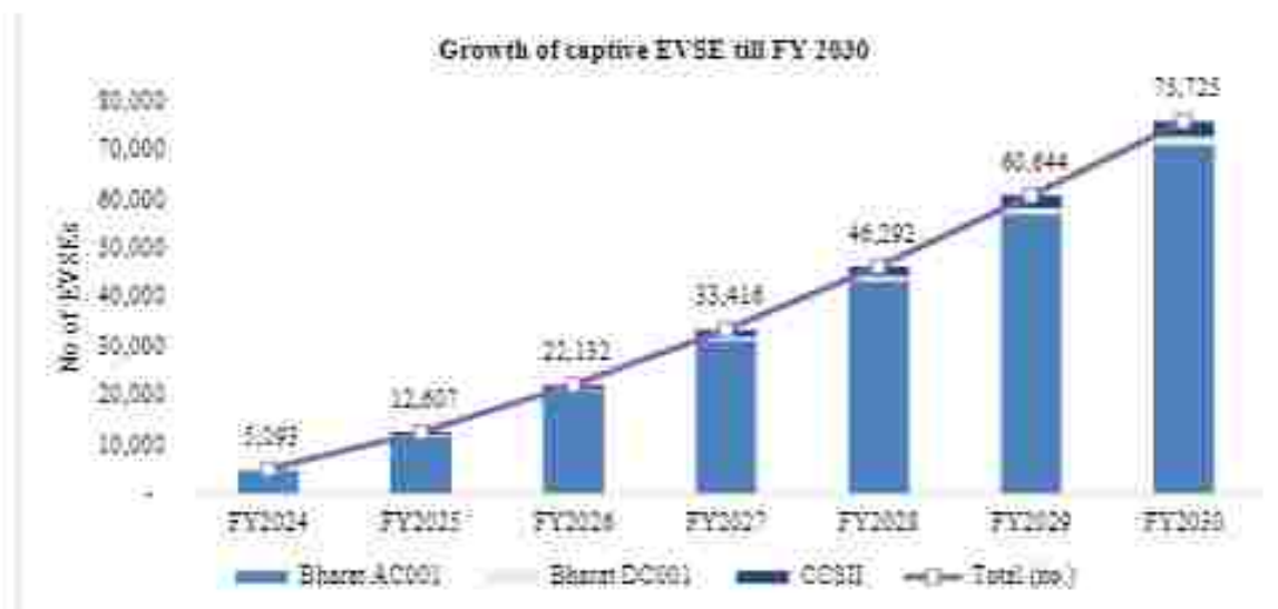
Graph 103: Projection of EVSE for Captive Charging stations
