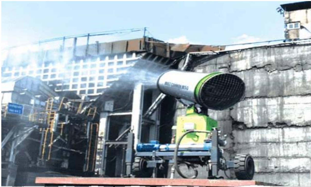
Fig. Mist Gun operation to control dust
