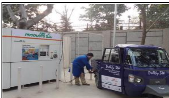
Figure 20. Hydrogen fuelled 3-wheeler developed jointly by IIT Delhi and Mahindra & Mahindra in New Delhi
