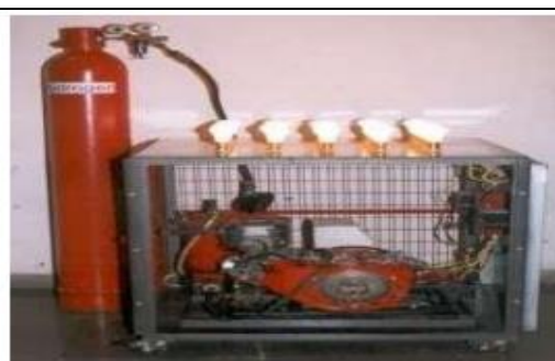
Figure 21. Total hydrogen S.I. engine genset using electronic fuel injection system
