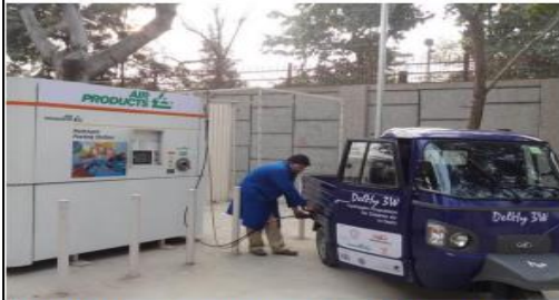
Figure 20. Hydrogen fuelled 3-wheeler developed jointly by IIT Delhi and Mahindra & Mahindra in New Delhi
