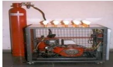
Figure 21. Total hydrogen S.I. engine genset using electronic fuel injection system
